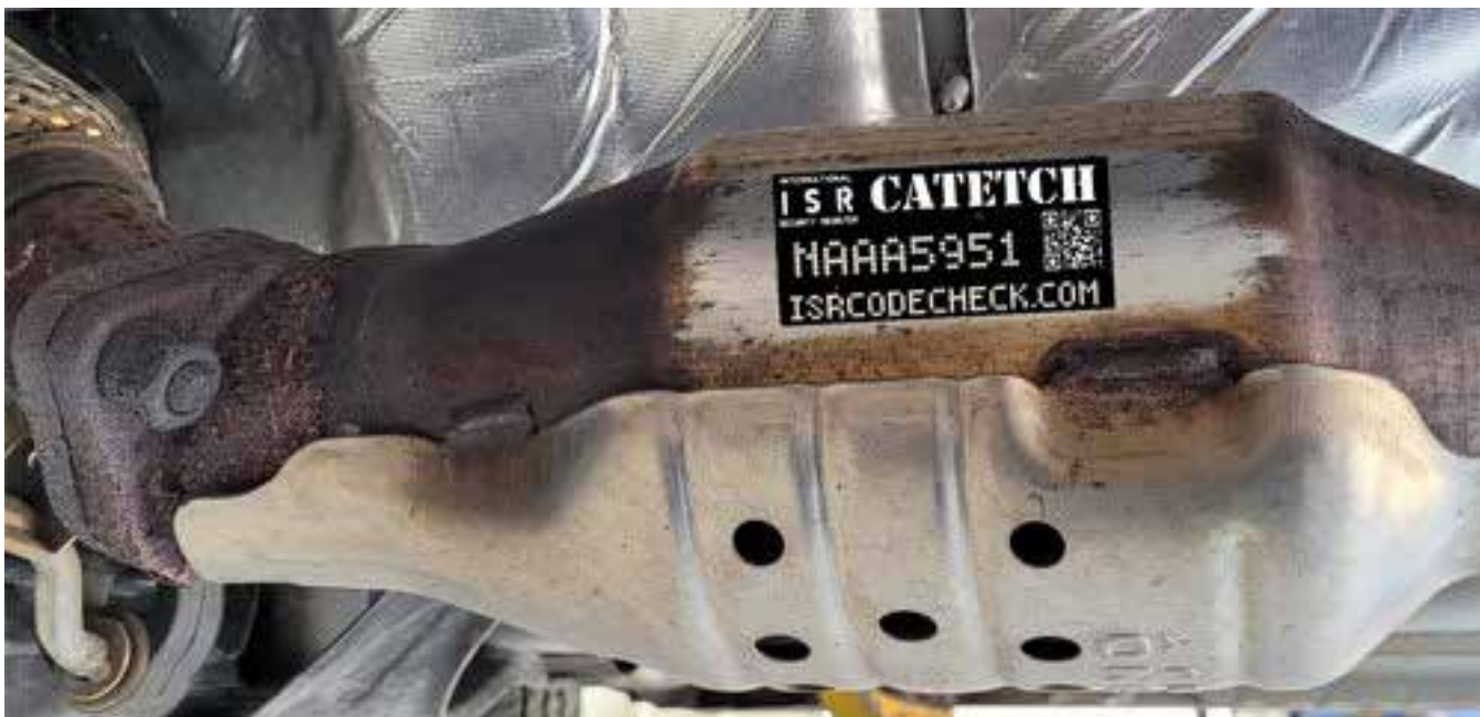
A catalytic converter is an exhaust emission control device that converts toxic gases and pollutants in exhaust gas from an internal combustion engine into less-toxic pollutants by catalyzing a redox reaction.
